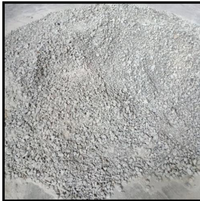
Figure 2: Coarse aggregate fraction 5 mm to 20 mm
